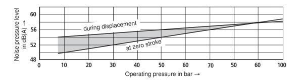
Measured in anechoic chamber to DIN 45635, page 26  $\,$
