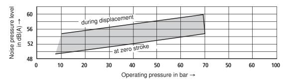
Measured in anechoic chamber to DIN 45635, page 26
