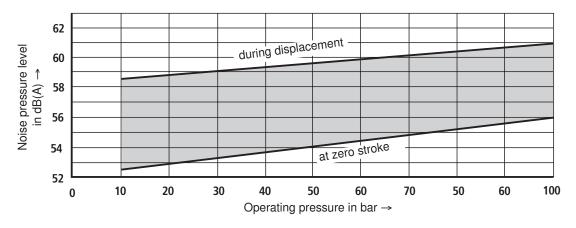
Measured in anechoic chamber to DIN 45635, page 26
