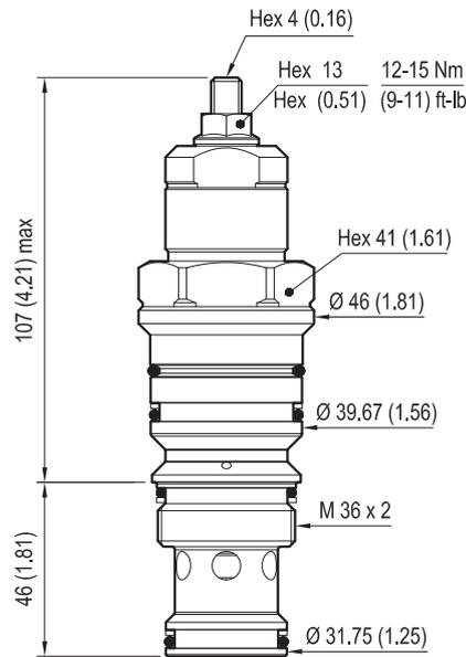
Turn adjustment clockwise to decrease setting and release load
