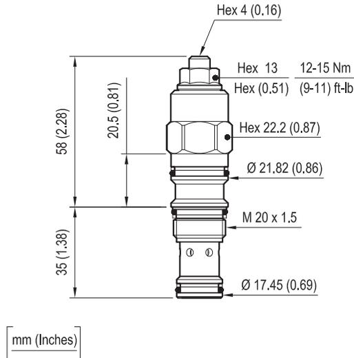
Turn adjustment clockwise to decrease setting and release load
