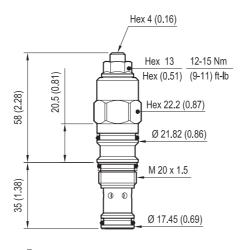
Turn adjustment clockwise to decrease setting and release load
