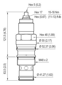
Turn adjustment clockwise to decrease setting and release load
