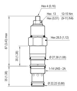
Turn adjustment clockwise to decrease setting and release load
