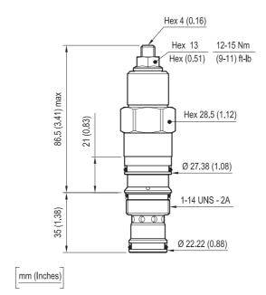
Turn adjustment clockwise to decrease setting and release load
