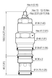
Turn adjustment clockwise to decrease setting and release load
