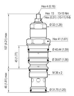
Turn adjustment clockwise to decrease setting and release load
